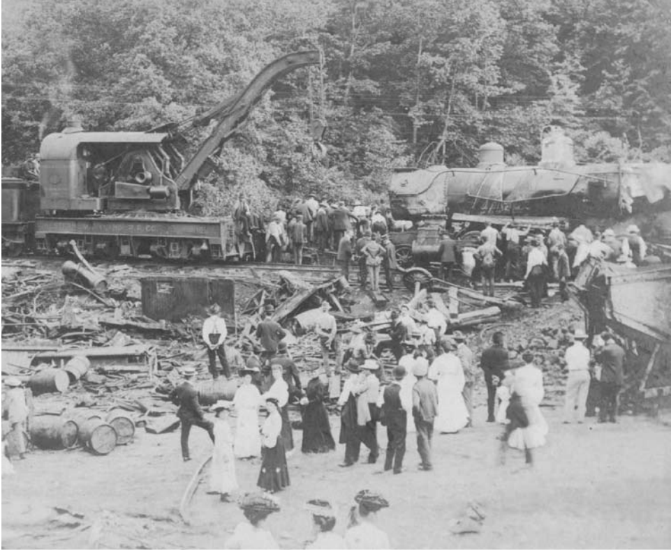
A steam crane clears the wreckage after two trains of the Western Maryland Railway crashed on June 17, 1905. (Western Maryland Railway Historical Society.)
